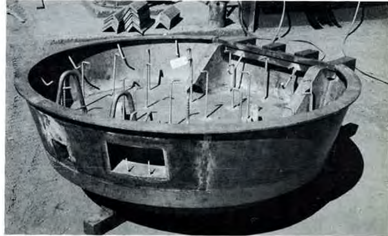
Fig. 34: Type SF 60 missile access doors with welded steel lifting hooks and hinges to specification of U. S. Army engineers. Steel rods are for holding concrete filling.
