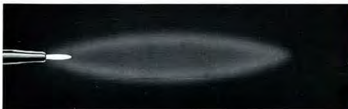
Fig. 20: A 50/50 mixture of oxygen and acetylene produces a neutral flame where the inside consists of a brilliant white cone \frac{1}{16} to \frac{1}{4} " long and the envelope flame is faintly luminous with a delicate bluish color.
