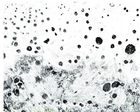
Fig. 2: Extensive carbidic area in a nodular weld indicating rapid solidification of the weld metal.
