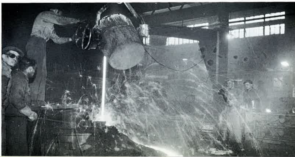
Fig. 31: Pouring the molten metal during welding by burning. Note the flow-off of metal used for promoting incipient fusion in the weld area.
