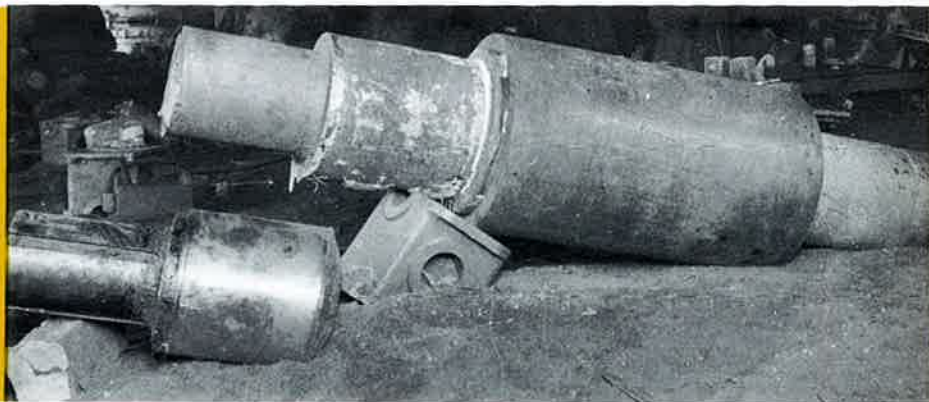
Fig. 29: Rubber roll after burning welding of new neck. Old broken neck in the foreground.
