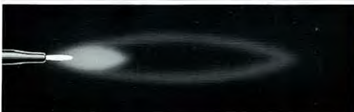
Fig. 21: The carburizing or excess acetylene flame consists of three zones. Between the inner cone and the bluish outer envelope there is an intermediate cone of whitish color. The length of this intermediate cone varies directly with the amount of excess acetylene.
