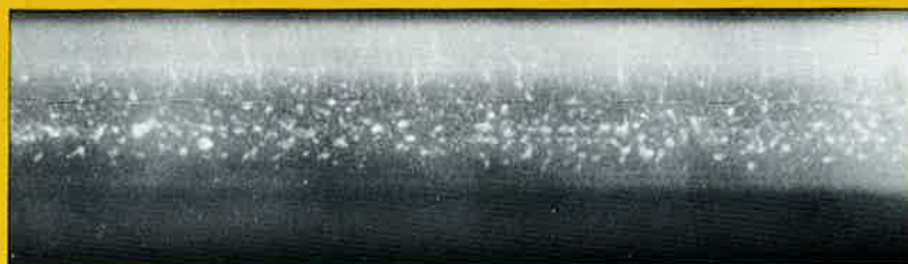
Fig. 15: Cracked weld shown by radiograph may have been avoided by preheat before welding.
