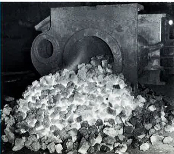
Fig. 28: Preheating marine cylinder prior to welding by burning. Repair approved by the Bureau of Shipping.
