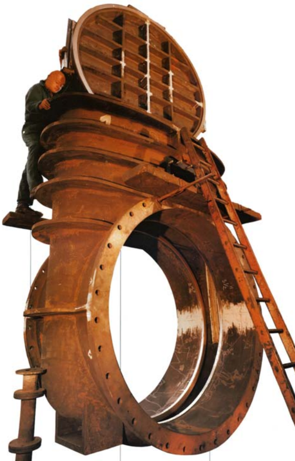
The body of this large wedge gate Valve, shown being assembled, is cast in MEEHANITE Type GD 35 and weighs over 9 tons. It features metallic sealing seat faces and a bore of 72 inch diameter. The valve has been installed for isolating duties in the cooling water circuit of a British nuclear power station.
