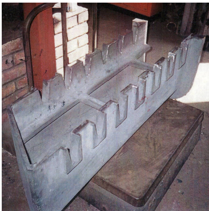
MEEHANITE Type CB 3 acid plant trough.
