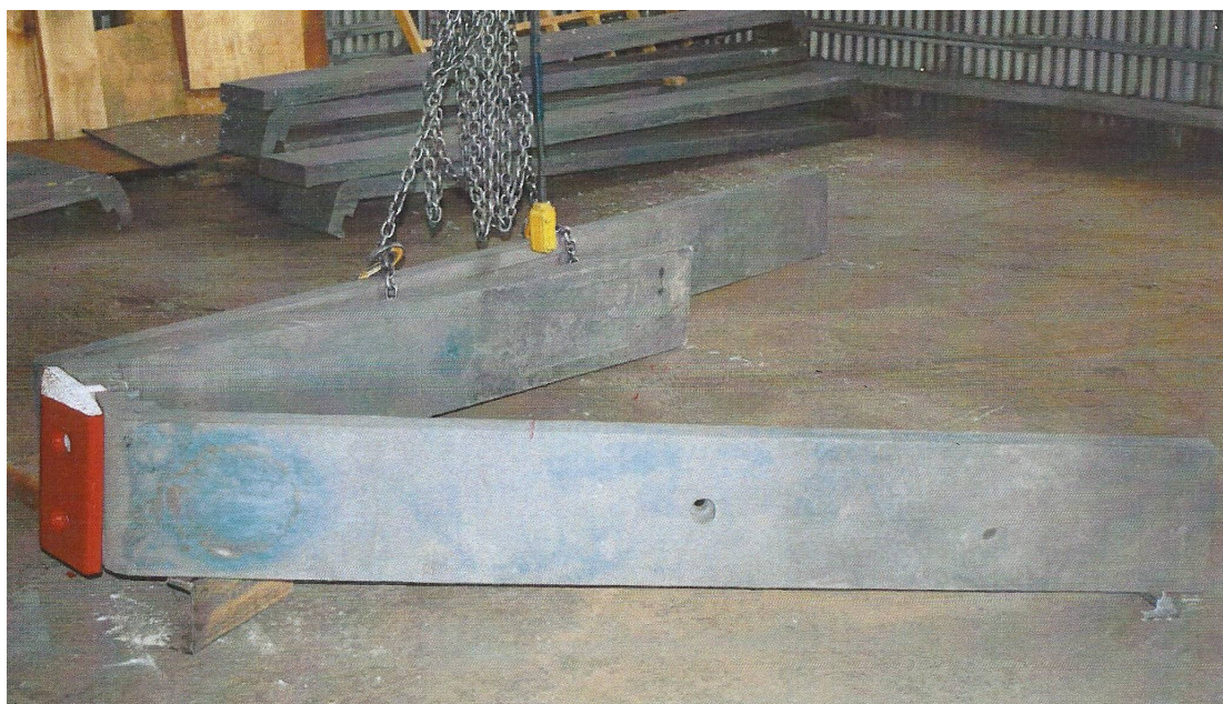
MEEHANITE Type W_{20} ore bin liners joined using a MEEHANITE Type SF400 cap.
